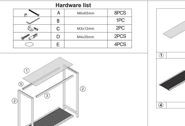
Do not tighten the screws fully during assembly. Fully tighten screws after the final assembly steps
