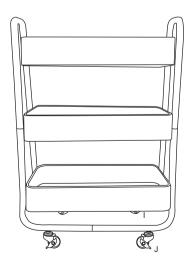
3. Assemble the bottom tray first, using (e)(f)(g) to connect the tray and tube frame together. Use the spanner (h) to fix the nut (g).
