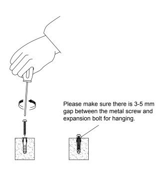
④ Install the metal screws into the expansion bolts. Please make sure there is 3-5mm gap between metal screw and expansion bolt for hanging.
