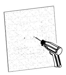
① Put the location holes card on the wall which you would like to hang the lamp. Use pencil or marker pen(not included) to locate 2 holes.
