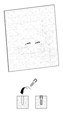
③ Insert the expansion bolts into the holes.
