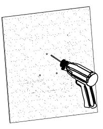
① Put the location holes card on the wall which you would like to hang the lamp. Use pencil or marker pen (not included) to locate 3 holes.
