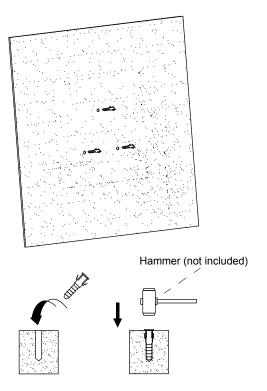
③ Insert the expansion bolts into the holes. Use hammer (not included) to make it smooth on the wall.
