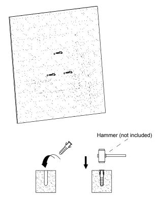
③ Insert the expansion bolts into the holes. Use hammer (not included) to make it smooth on the wall.
