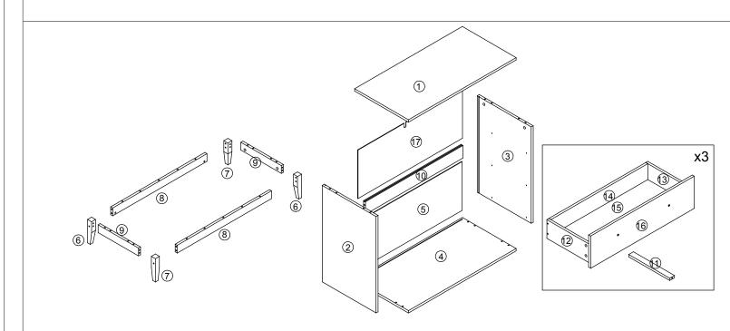
Do not tighten the screws fully during assembly. Fully tighten screws after the final assembly steps.
