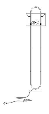
④ Install the bulb - Max. 40W (not included) into the lampholder. Check to ensure that all the components have been assembled correctly. Connect to the mains supply
