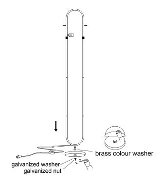
①Assemble the metal tubes as above manual.
