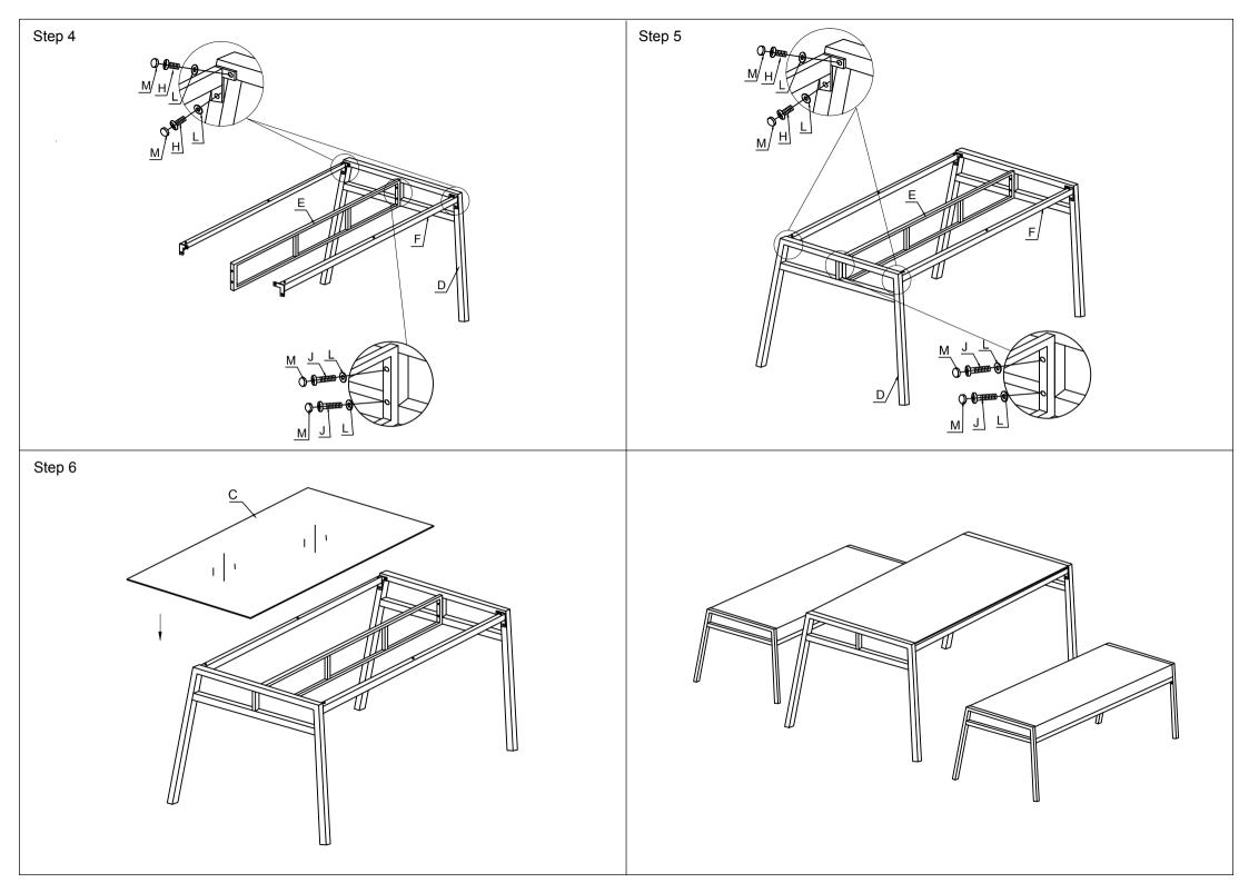
ATTENTION: DO NOT TIGHTEN THE SCREWS FULLY DURING ASSEMBLY. FULLY TIGHTEN SCREWS AFTER THE FINAL ASSEMBLY STEP.
