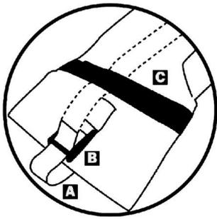
3. Run the straps(A) through the buckles (B) on the opposite side of the vehicle and pull VERY tight to secure the rack to the roof.
