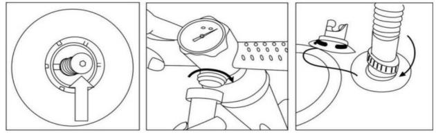
A).Unscrew the valve cap and press down on the pin to open the valve. Let the air flow naturally into the product, then press down on the pin again to close the valve (in the UP position).
