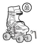
2. Separate the boot and the chassis.
