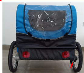
6. Install the cover with snaps and velcon closures around the hood, which marked with red arrows(pic2 and pic2-1), after that tighten the tie of pic3
