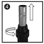
Loosen (anticlockwise) the post height adjustment Locking Ring, pull out the inner chrome tube to the desired height and then retighten the locking ring.
