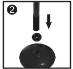
Insert the Plastic Collar into the top of the plastic base cover. Insert the bottom of the Stand Post into the collar.
