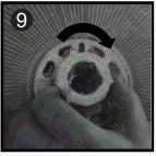
Fix the back safety grille into position by screwing the Locking Nut (clockwise) tightly by hand. (Note: Do not over tighten the locking nut.)
