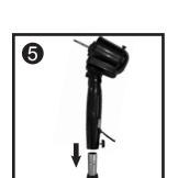
Place Motor Assembly at the top of the Stand Post and lower down all the way.
