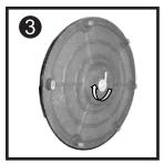
Tilt the Base and place the Weight in the centre of the base. Fasten in place by use of the Locking Lever and Washer and tighten.
