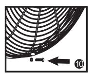
Using the small screw and nut, fasten the two grilles together.
