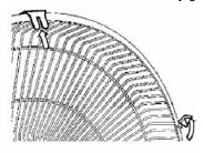
Place the front safety grille into position by positioning the locating tab at the top of the grille (above image) over the top of the rear grille and then secure the grille by closing the clips over the outer rim (below image). The screw and nut at the bottom of the grille must be fitted.
