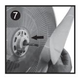
Place the **Fan Blade** onto the motor spindle.
