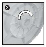
Flip over on its side. screw on the **Plastic Nut** (clockwise) and tighten. Do Not overtighten.
