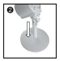
Place the round **Base** on a flat level surface and then insert the end of the post through the hole.
