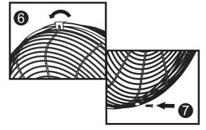
Place the **Front Safety Grille** into position and secure it by closing the clips over the outer rim.
