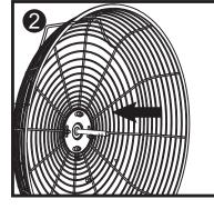
Fit the **Back Safety Grille** into position and refit the 4 Screws and tighten. (\*Note: The handle on the back of the grille should be at the top)
