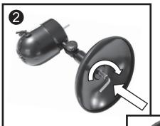
Insert the threaded part of the "L" screw through the hole in the bottom of the base and screw all the way in tightly.
