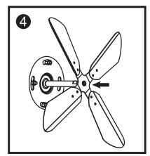
Slide and push the **Fan Blade** onto the spindle. Push on until the end of the fan blade hole is aligned with the end of the spindle.
