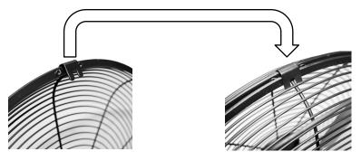
Secure the grille by closing the clips over the outer rim.
