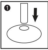
Locate the neck of the Fan Head into the recess in the top of the Base then flip over.
