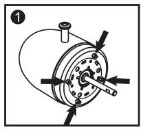
Remove the protective plastic sleeve from the motor spindle shaft and the 4 Screws as identified.
