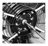
If fitted, remove the protective plastic sleeve from the motor spindle shaft and discard it.
