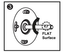
Rotate the motor spindle until the "FLAT" surface is facing up.
