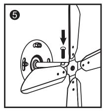
Then fix and tighten the screw. (Note: Ensure the screw is lined up with the "FLAT".)
