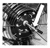
Slide the fan blade onto the spindle shaft ensuring the screw is lined up with the "flat" surface on the spindle shaft as shown.
