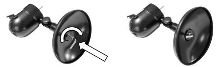
Stand the Fan assembly upright on its base ready for assembling the grille.
