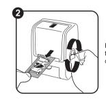
Feed the paper strip through the machine, turn the dial knob clockwise until the paper comes out to the other end.
