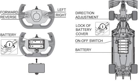
Function: Forward, Reverse, Turn Left, Turn Right. Features: Authentic car styling with injection moulded body, independent suspension system.
