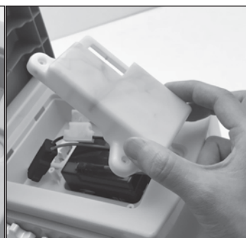
4. Unscrew the three screws on the battery compartment with a screwdriver and remove the battery retainer.
