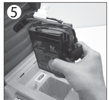
5. Carefully lift the old battery and replace it with a new battery.
