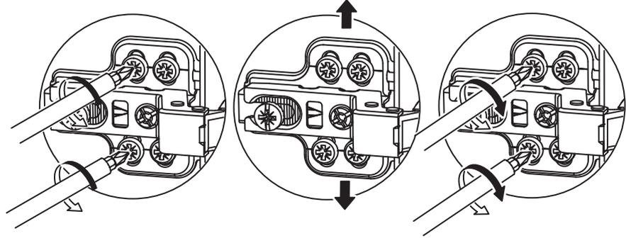
1. Loosen the two mounting screws on both hinges, but only slightly. ...
