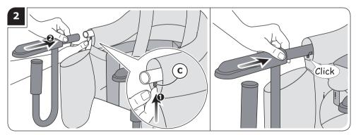
Press Shrapnel (C) and simultaneously put the clamp assembly into the Back Tube (B) until there is a "Click" sound. Make sure the side slot of the clamp tube is faced outwards during assembly. Repeat for both sides.
