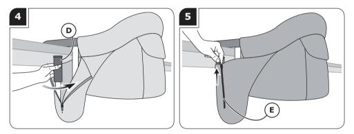
Screw Adjustor (D) upwards to secure to the table surface tightly, then zip up the part (E). Repeat for both sides.
