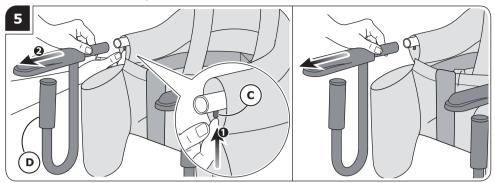
Release the Shrapnel (C) and simultaneously pull out the clamp (A) from the tube. Repeat for both sides.
