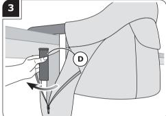
Unscrew the Adjustor (D) to loosen the clamp.
