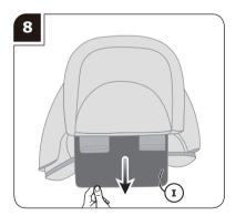
Unfasten the fastening grips underneath and take out the Seat Pad (I) from the Seat Cover (H) as per image.
