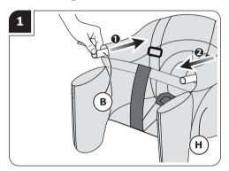
Insert back tube (B) into the sleeve of seat cover (H).
