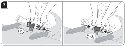
Insert the side clips into the main buckle (F). You will hear a "Click" sound when the buckle is in position.
