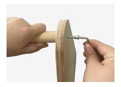
Put one end of the wooden pole to the hole on panel then take the screws and pass them through the hole, using the allen key to tighten.
