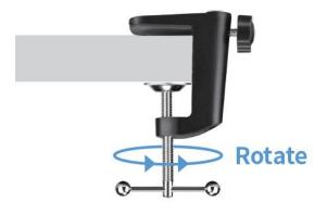
Step 2: Fix the microphone stand on the base, and rotate the nut to fix the stand.
