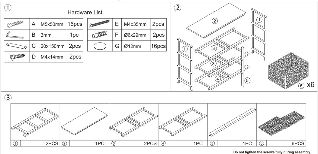
Fully tighten screws after the final assembly steps
