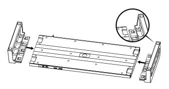
2)Pull the stands into the back of the platform and make sure the stand
