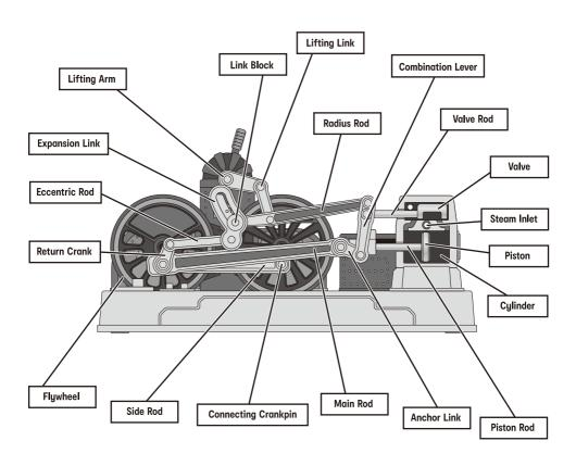
The relationship between steam, valve, piston and wheel in a real steam engine are described as below:
