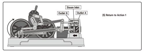
In this design, the upcoming pressured steam can push the wheel and as a result move a train.
