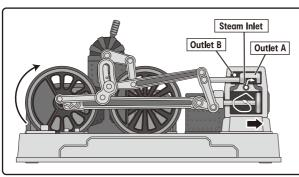
(4) As the valve moves to the right side, the steam starts to come into the cylinder from the steam inlet. Outlet A closes.
