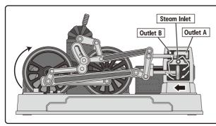
(1) As the valve moves toward the right, the steam comes into the right side of the cylinder from the steam inlet.
