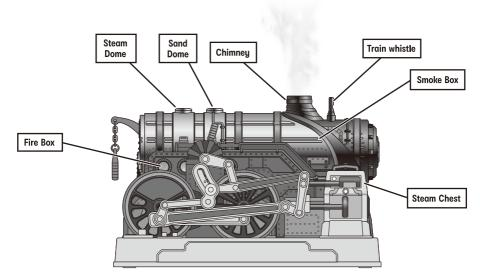
Fire Box: A furnace chamber. Coal will be added into the fire box for fire. The fire will heat up the water in the boiler. After the water is boiled, steam comes up and goes through pipes.
