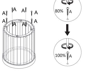
ATTENTION: PLEASE LOCK A SCREW AT 80% BEFORE ALL THE HOLES ALIGNED, THEN TIGHTEN ALL SCREWS AT 100%.
