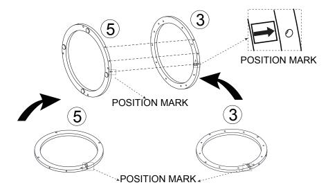
ATTENTION: CHECK THE POSITION MARK ON THE BOARD. THEN ALIGN MARK AND ALL SCREW HOLES ON 3&5.
