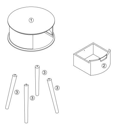
DO NOT TIGHTEN THE SCREWS UNTIL THE PRODUCT IS FULLY ASSEMBLED.
