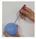
To replace batteries, use a pencil or other pointed object to push out the old batteries.
