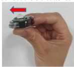
Insert 2 new CR2032 batteries with "+" sides matching the orientation shown.
