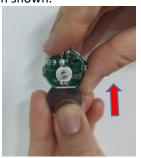
Push the LED module back into the bocce ball cap by aligning the black tabs on the LED module with the two openings on the cap as shown. Then screw the cap back onto the bocce ball and tighten it firmly. It is normal that you find the screw can still turn after tightening.
