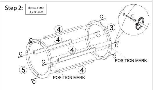
ATTENTION: LOCK PART 4 WITH C SCREW AND KEEP ALL SIDE SCREW HOLES. POSITION MARK ARE ALIGNED.
