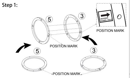
ATTENTION: CHECK THE POSITION MARK ON THE BOARD. THEN ALIGN MARK AND ALL SCREW HOLES ON 3&5.
