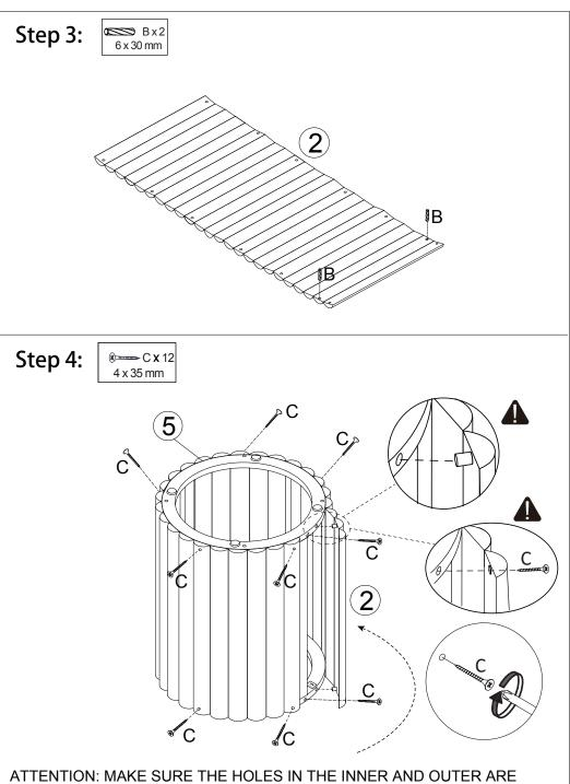
ALIGNED, AND THEN C SCREW ARE TIGHTLY LOCKED IN SEQUENCE.
