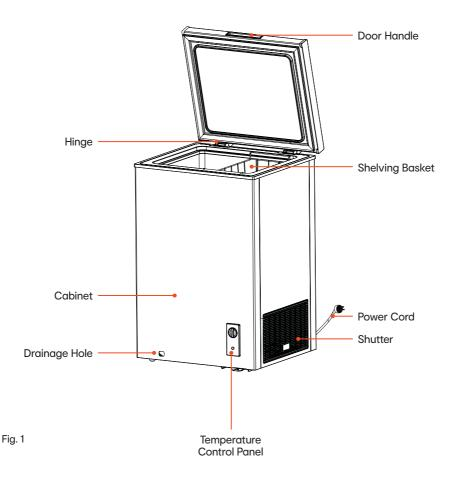
**NOTE:** After long term use, there maybe a certain degrees of wear with the hinge, causing a noise when opening or closing the door, reducing the service life of hinge. It is recommended to regularly put the grease on hinge for maintenance as it can effectively eliminate noise and extend the service life of the hinge.
