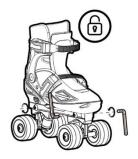
2. Separate the boot and the chassis.
