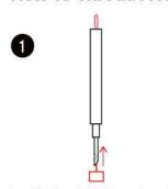
Insert the threader into the punch needle from the needle point and completely through the barrel until it comes out the opposite end of the tool.
