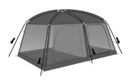
Draw out the fiberglass pole from pole sleeve. Then pack back all poles and tent body into bags.
