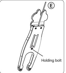
2. Attach the frame to the front fork by Inserting the Frame into the front fork.
