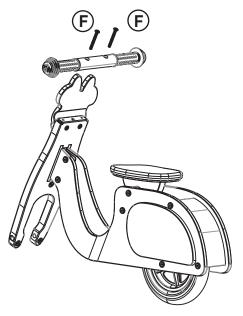
4. Insert 2 pcs of Spacer Nuts (part I) into the center of bearings.
