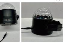
4.Plug the USB cable into a free USB port or USB wall charger with 5V 1A output. Use the remote control to control the disco ball.
