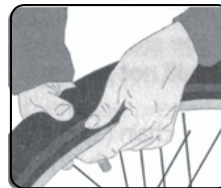
FIGURE F Use thumb to press valve stem through hole in rim. Make certain valve stem is straight.
