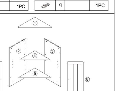
DO NOT TIGHTEN THE SCREWS UNTIL THE PRODUCT IS FULLY ASSEMBLED.
