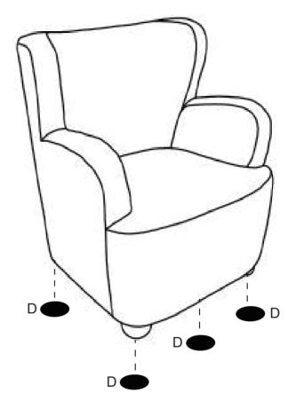
If the chair is not smooth after assembly. please use the part D to stick on the bottom of the foot to level.
