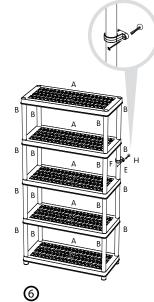
To fix onto the wall, place the wall mounts to the pillars of the shelf. Screw wall anchors into place. Then, insert the screw and tighten.
