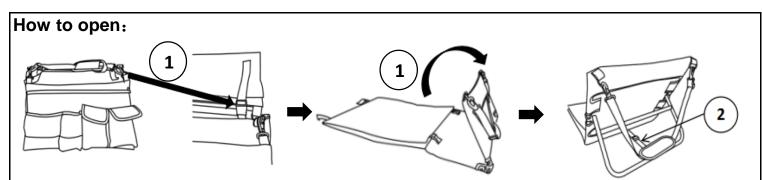
OPEN 1. Open the buckles on both sides, and open the back tube.
