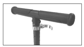
Step 3: Press the stem pin and choose a suitable position and then close the quick release.
