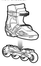
4. Tighten the screws on the new chassis.
