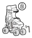
2. Separate the boot and the chassis.
