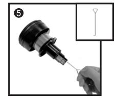
Use the supplied **Wire Hook tool** to remove any hair or fluff etc. from the cavities, then wipe over with a very lightly moistened (not wet) clean cloth and mild detergent. **DO NOT wash it as there are electrical contacts inside this part.**
