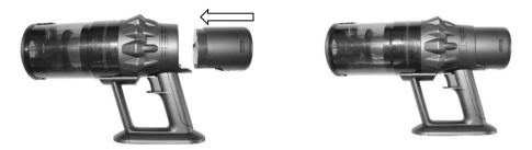
Other than for maintenance, there should be no need to remove the battery pack once fitted, however, when you do need to remove it, press the release button located underneath the battery pack, and at the same time, slide the battery straight out.
