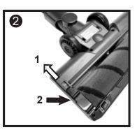
Slid it back to unlock the **Rotary Brush** Holder. The holder will pop up when released. Grasp the **Rotary Brush** and lift it up and out.
