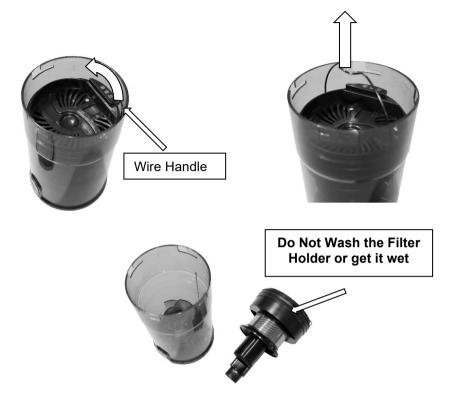
Only wash the filter if it is very dirty, otherwise, just tap the edge of the filter on a hard surface to dislodge any dust and debris.
