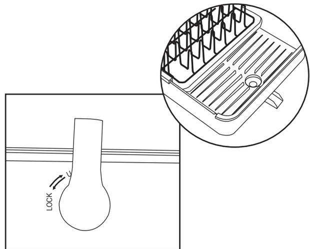
Turn to unlock the draining spout underneath the tray.
