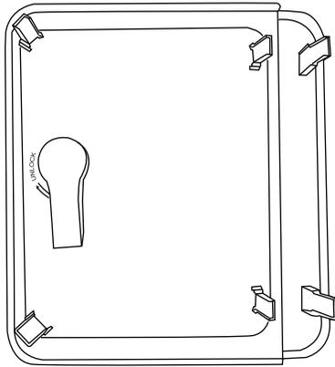
Unfold the six supporting feet at the bottom of the tray. Ensure all feet are securely extended to provide stability.
