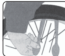
FIGURE B Lift bead with spoons or tyre tools.
