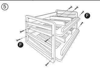
Note: If the bottom is uneven during installation, use a wrench to adjust the screw tightness to level it.
