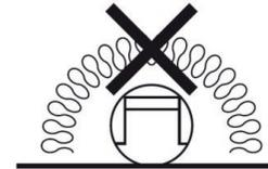
The LED driver that can be used where normally flammable materials. Including building insulation, are or may be present, but cannot be abutted against any material and cannot be covered in normal. Minimum clearance distance from the top and sides of the control gear to normally flammable building element is 75mm; as shown in below picture, A=B=C=Min.75mm.
