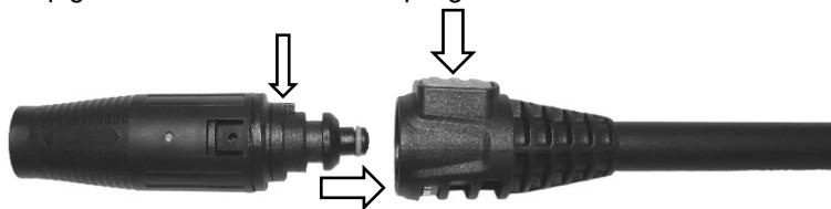
Press the Locking Button on top of the Wand and at the same time, push the Variable Spray Nozzle onto the Wand then release the button to lock the Nozzle in place.
