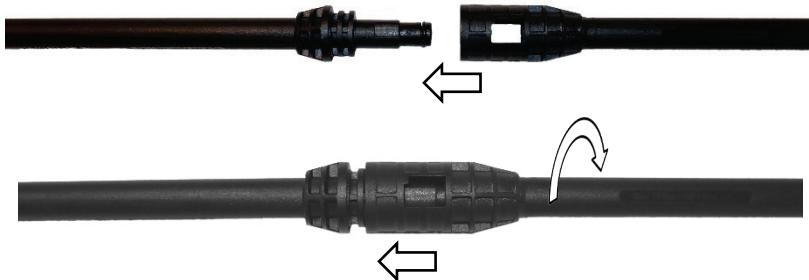
To remove the Extension Wand, push the Gun onto the Extension Wand, rotate the Gun anticlockwise, then pull the two components apart.
