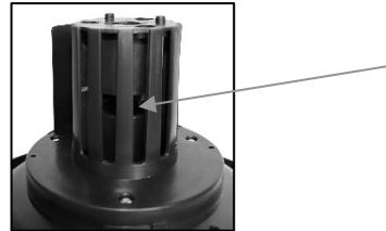
This float is designed to rise up with the water level inside the dust canister and will block off the air inlet into the suction impeller.
